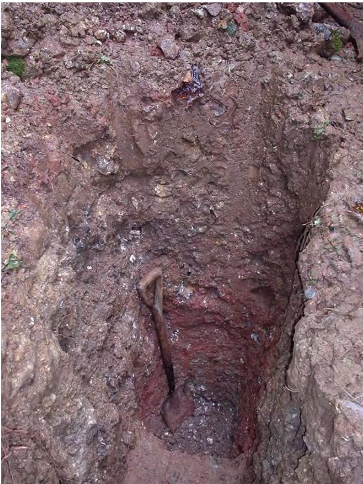
**Figure 3 (above): 1.5m trial pit by garage – shows flints in red, becoming purple with depth, clays**
